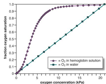
**Figure 13.1** Solubility of gaseous O<sub>2</sub> in water and hemoglobin solutions. The units of oxygen concentration in the air over the liquids are kilopascals (kPa). Original Art with help from Durwin Striplin, Davidson College Chemistry Dept. Raw data from Severinghaus, 1979, his table I.
