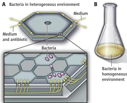
**Microenvironment for bacterial evolution.** Fabricated microenvironments, such as the microfluidic device described by Zhang *et al.* (A), may provide a relevant approach to understanding microbial evolution in real-world environments that are spatially complex and full of chemical and nutrient gradients, and so differ from homogeneous liquid cultures (B).
