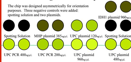
This design was then spotted on a DNA chip using a Microarrayer. The colors above indicate a possible result after the chips have been scanned.
