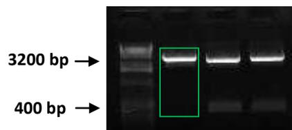
**Figure 14. Digestion with AsiSI shows that Cre's internal AsiSI site has been removed.** Minipreps were digested with AsiSI only. As seen in colonies 2 and 3, there was a band at 400 bp if the internal restriction site was still present. If there was no internal restriction site, AsiSI cut once, producing a single band at 3200 bp, as in colony 1.
