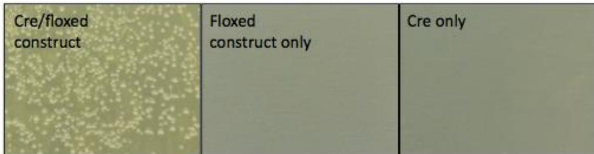
**Figure 18. Cotransformation of Cre and the floxed construct does not result in reporter output.** Chloramphenicol/ampicillin plates transformed with only Cre or the floxed construct produced no colonies. Cotransformation of these two plasmids is essential for colony growth. All cotransformed colonies with the RFP reporter were white.
