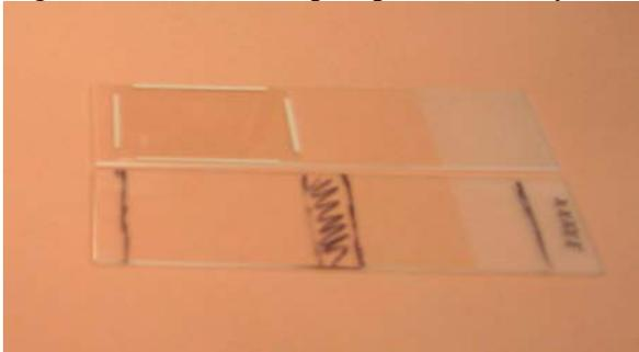
10. Place the slide into either a slide hybridization chamber or a 50 ml conical tube. Be sure to include some water in either case to keep the hybridization mix from evaporating (the chambers have wells that hold ~20  $\mu\text{l}$  of water; for the conical tube, just add ~50  $\mu\text{l}$  to the tube).
