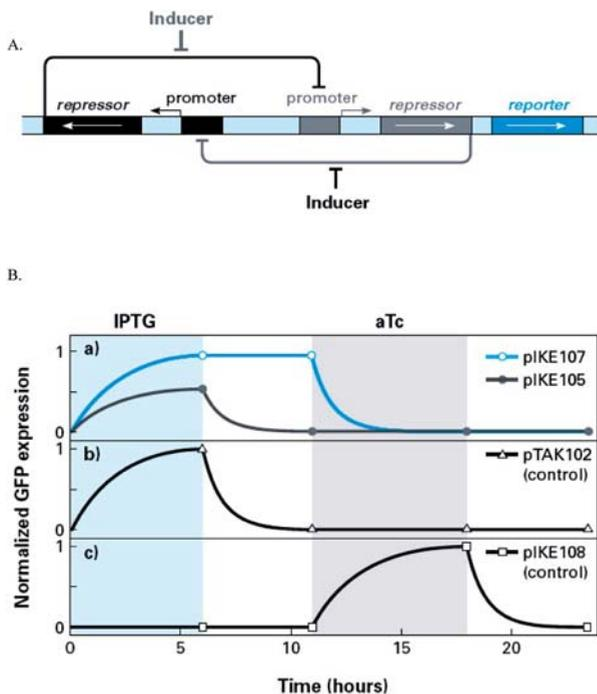
**Figure 2.** Bistable toggle switch. A. Generic design of a bistable switch that can be flipped one of two ways depending on which inducer is applied. B. Data produced by the final bistable toggle switch (panel a, blue trace) as well as several control constructs (black traces).
