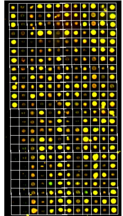
At any time in the gridding process, you can mouse over a spot and identify its location (x and y coordinates in pixels, row, column and spot number) as well as its identity from the gene list. This information is displayed in the bottom left corner and is especially useful for navigating during segmentation.
